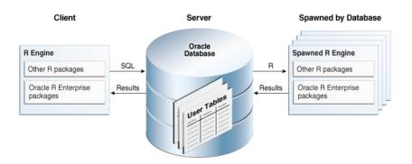
Oracle R Enterprise Components: Client R Engine, Database server Engine, and R Engines spawned by the database.
